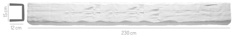
*False wooden beam with U section that allows finishing your ceiling or wall if matched to the JUGLA strip. Important could be the surface finishing that can be obtained through painting.*
